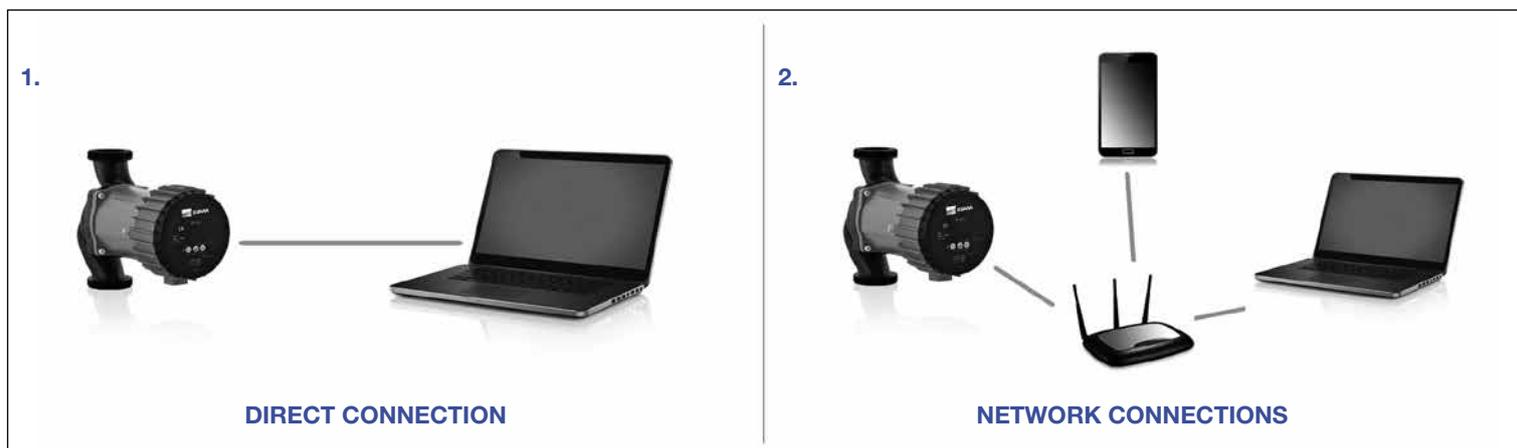
Once you have completed the Ethernet connection, you can access the circulator using any internet browser (Chrome, Internet Explorer, Firefox, etc.) typing in the IP address of the pump, indicated in the manual. Once you have completed the connection to the PC, various video pages enable you to fully program the circulator, the digital inputs, the relays etc. and also to display the instant operating parameters, the power consumption and the errors.
